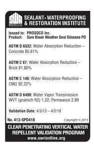
**NOTE:** The SWR Institute Validation Program uses standardized testing for validation purposes, including testing on CMU. PROSOCO <u>does not</u> recommend the use of Siloxane PD on CMU. Please reference the Substrate Chart on page 2.
